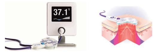
**Figure 1** SpotOn<sup>TM</sup> system and zero-heat-flux (ZHF) technology. The thermal insulator and warming circuit are used to eliminate the flow of skin-surface heat to the environment, establishing conditions in which the temperature gradient should be zero between the thermistor on the skin surface of forehead and deep tissue. Core temperature rises the surface through isothermal pathway. Figures are reprinted with permission from 3M.
