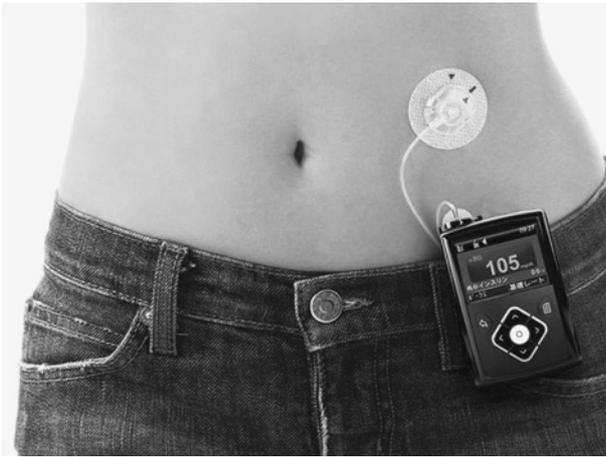
Fig. 6 Artificial pancreas (MiniMed 620 G, Medtronic MiniMed, Inc)<sup>13)</sup>
